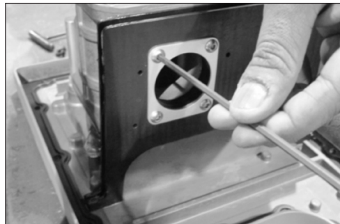
Figure 9.37 - Remove 4 (#10-24) screws on main gasket
