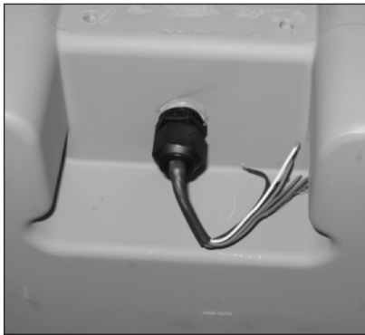
Figure 7.15 - Pulse output cable on backside of meter
