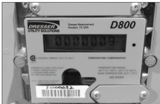
Figure 6.1 - Label on D800 meter
