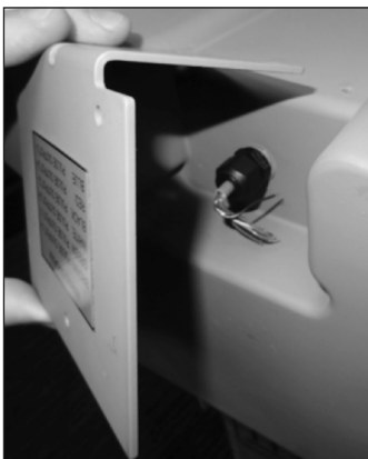
Figure 7.28 - Pulse output cable is covered by a protective plate
