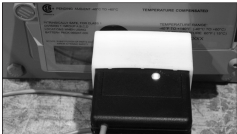
Figure 10.17 - Light indicating connection established
